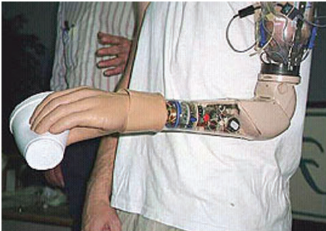
Fig 5- Utah Arm 3 with Connector Options for Separate Elbow and Hand Inputs
