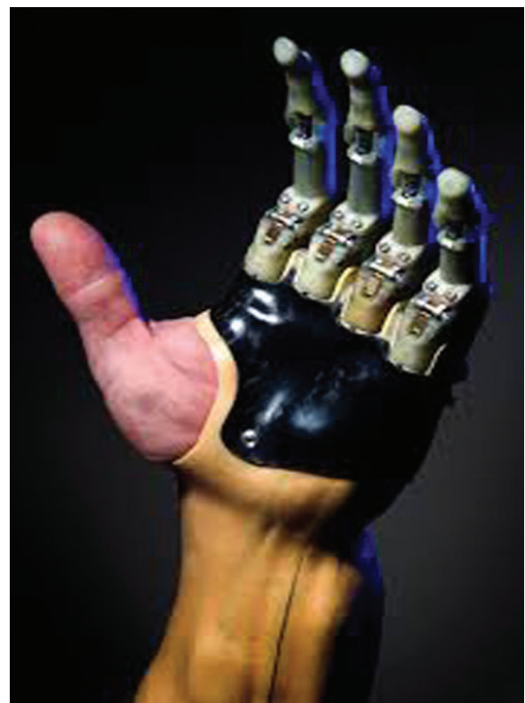
Fig 8- Myoelectric Prosthetic Partial Hand Fingers
