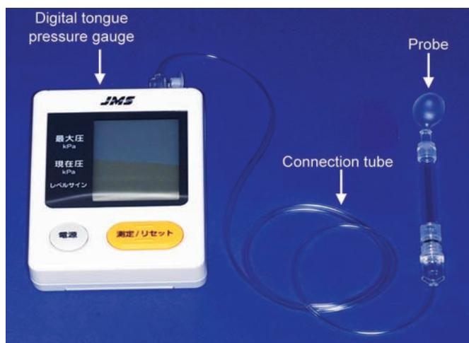
Fig. 1: The digital tongue pressure gauge and probe
