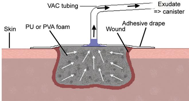
Fig. 1: Schematic diagram showing a cross-section of wound with VAC dressing
