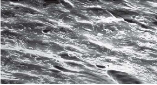
**Fig. 5.** Scanning electron micrograph of MicroPores implant interface. Surface may be blasted with hydroxylapatite and chemically milled for greater cell adhesion
