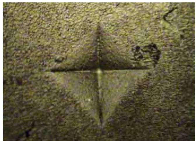
Fig. 6: Microscopic image of indentation at 40× magnification
