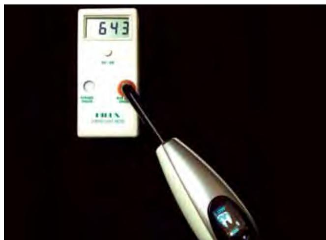
Fig. 2: Radiometer showing the light intensity
