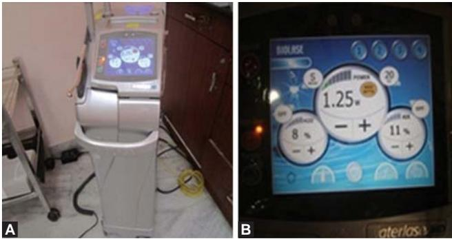
**Figs 1A and B:** (A) Er,Cr:YSGG laser (Biolase™ Waterlase MD), (B) panel setting [1.25 W average power and 20 Hz (62.5 mJ/pulse)]
