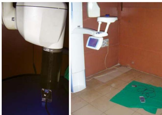
**Fig. 1:** Calibrating exposure dose from IOPAR and OPG machine using Unfors Multi-O-Meter
