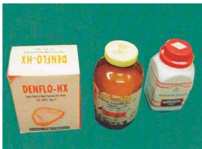
Fig. 1: Materials used for experiment (Type V Dental Stone, calcium hypochlorite, magnesium chloride)
