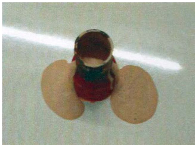
Fig. 2: Test of consistency by measuring the length of slump
