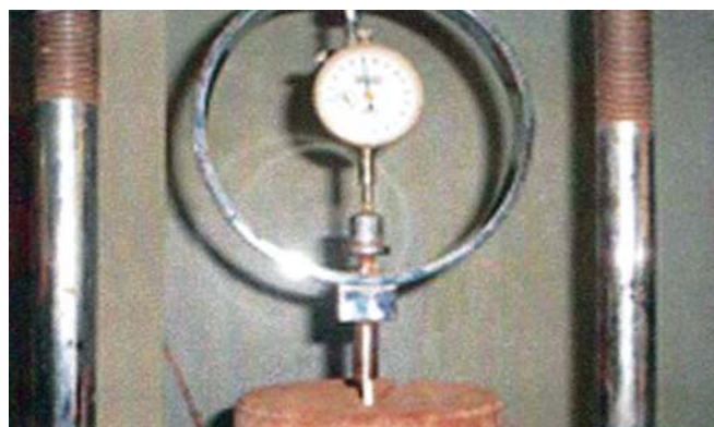
Fig. 9C: Compressive strength testing with dial gauge attached
