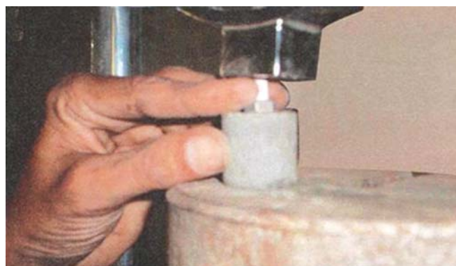
Fig. 9B: Close view of vertical placement of specimen.
