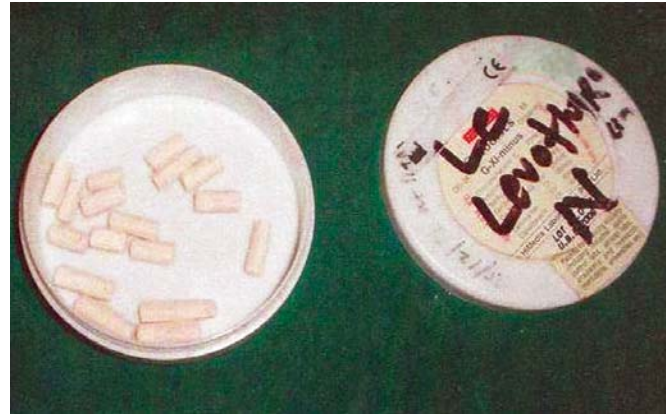
Fig. 6: Specimens prepared of type V dental stone and its incubation
