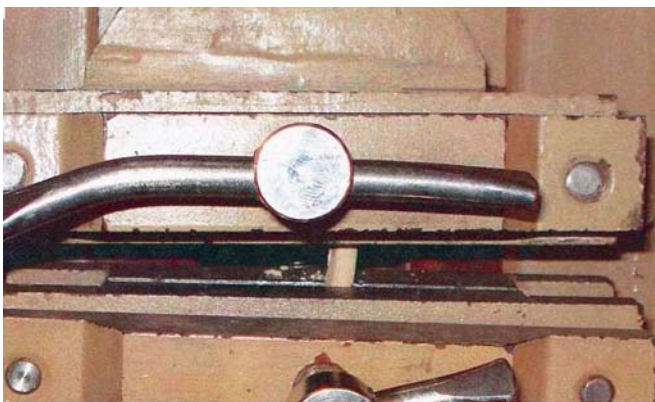
Fig. 10B: Close view of specimen, placed inside Tensile strength tester
