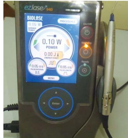
Fig. 3: Soft tissue Diode laser unit with 940 nm wavelength
