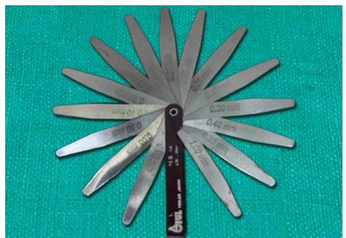
Fig. 5: Feeler gauge to measure the amount of separation at tooth contacts
