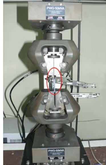
**Fig. 3:** Bracket archwire assembly mounted on universal testing machine
