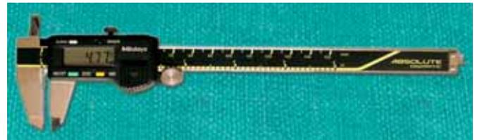
Fig. 2: Digital Vernier calipers
