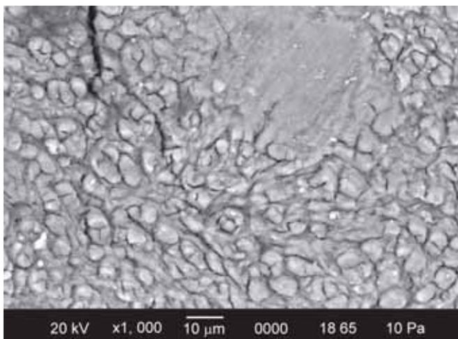
Fig. 2: Diode laser exposure for 30 seconds
