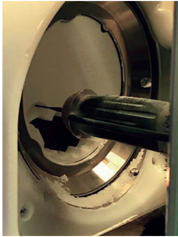
Fig. 11: Milling of the restoration
