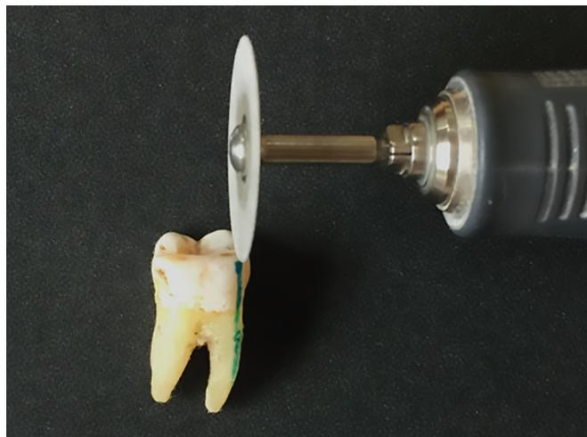
Fig. 1: Photograph showing 1 mm sample preparation using carborundum disk
