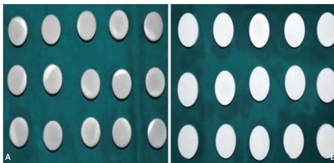
**Figs. 2A and B:** SLA treated (A) titanium specimen (A<sub>2</sub>), (B) zirconia specimen (B<sub>2</sub>)
