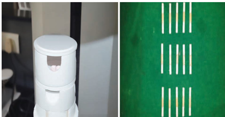
Figs 4A and B: (A) Sintering machine; (B) Finished zirconia specimens
