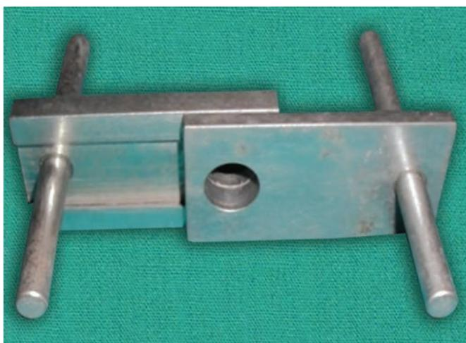
Fig. 1: Customized sliding jig assembly
