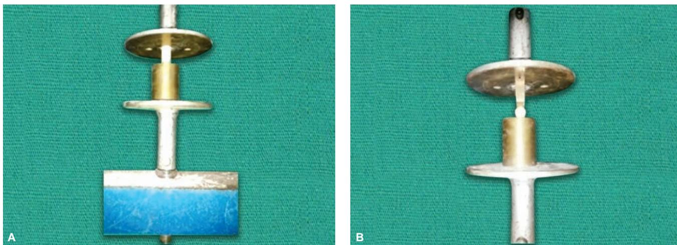
**Figs 3A and B:** Samples were attached to universal testing machine for evaluation of compressive and diametral tensile strength
