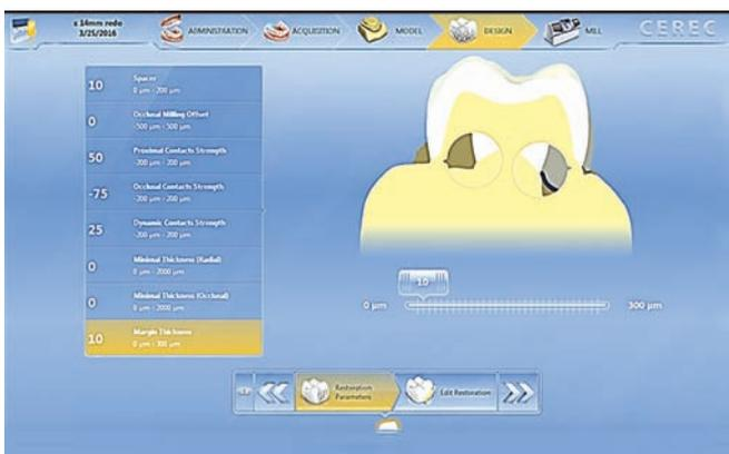
Fig. 4: Restoration parameter for the cement spacer was set at 10 microns for all specimens
