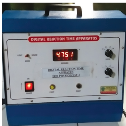
Fig. 1: Digital reaction time apparatus operator (investigator) side
