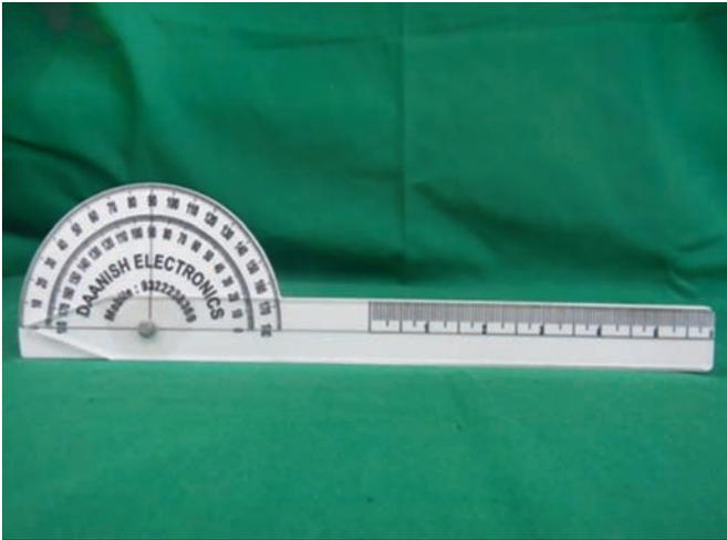
Fig. 2: Modified goniometer: front view
