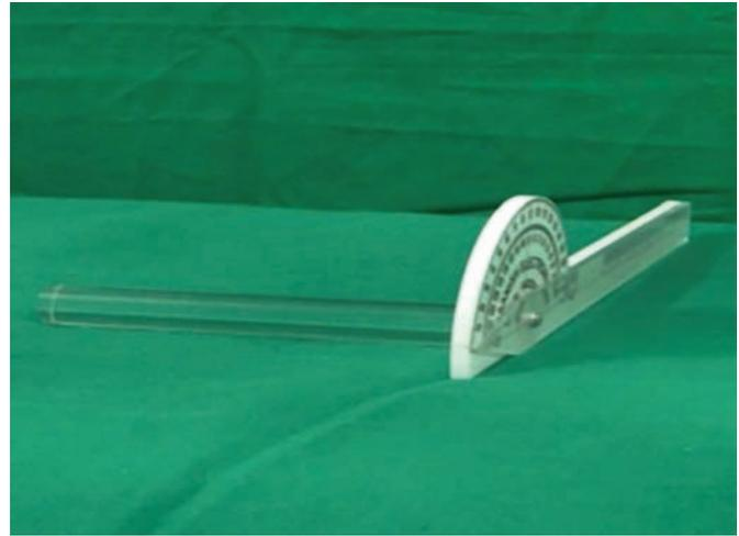
Fig. 3: Modified goniometer: oblique side view
