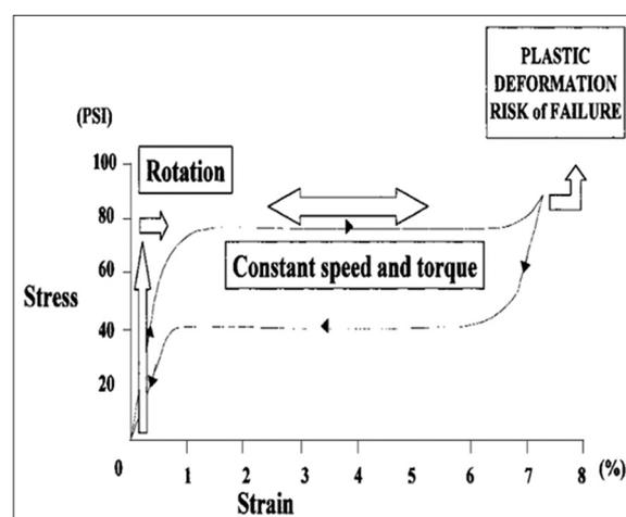
Figure 2: Super elastic behavior of NiTi alloy
