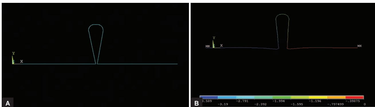
Figs 3A and B: Teardrop loop without preactivation bends. (A) Base model, (B) Model after 4 mm activation
