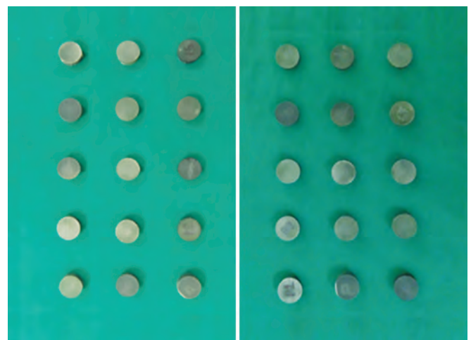
Fig. 1: Samples of laser-sintered Co-Cr disks
