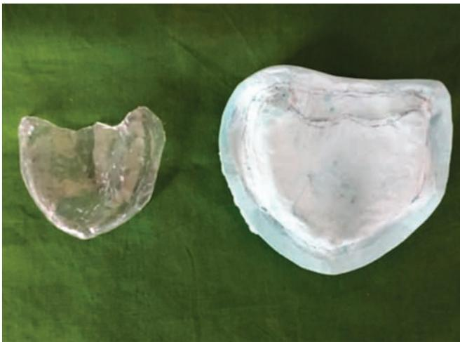
**Fig. 3:** Polyethylene sheet vacuum pressed over master cast
