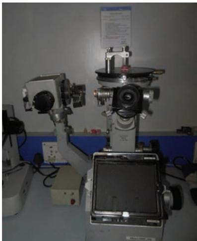
Fig. 3: Vickers hardness test
