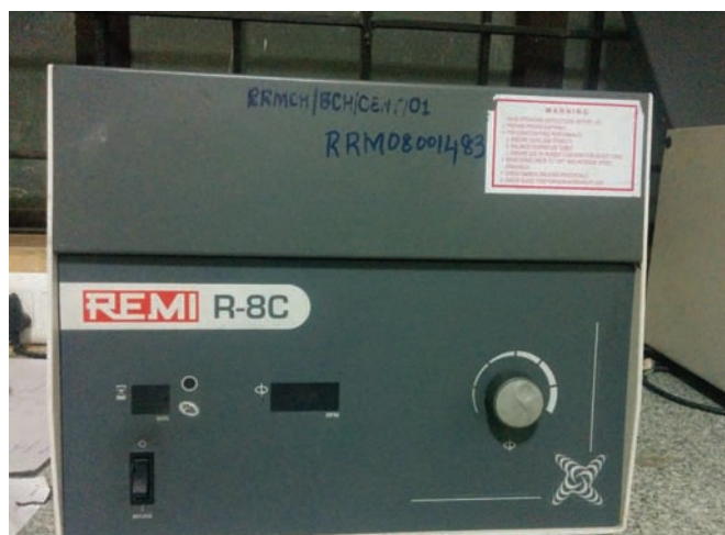
Fig. 1: Centrifugation machine REMI R-8C used for PRP preparation by double spin method
