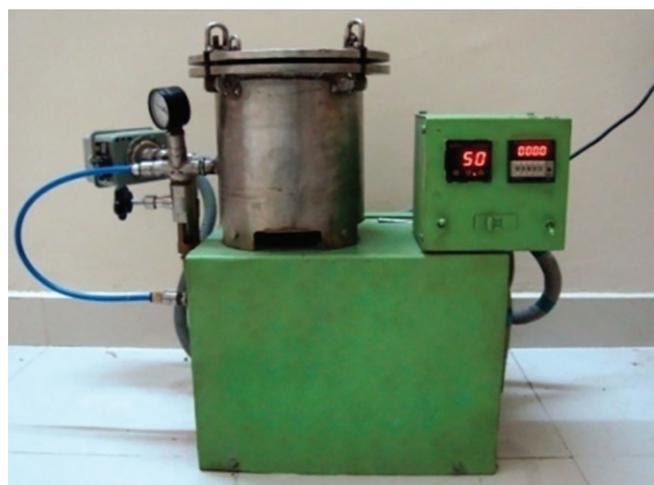
**Fig. 2:** Custom-made pressure pot
