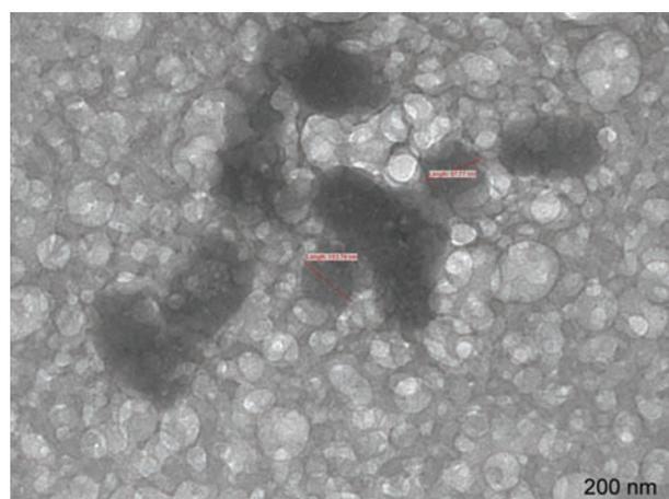
**Fig. 2:** The TEM micrograph of cerium NPs synthesized by seed extract of *P. vulgaris*. The CeO<sub>2</sub>NPs shown in the micrograph are in the range of 97 to 103 nm in size (scale at 200 nm)
