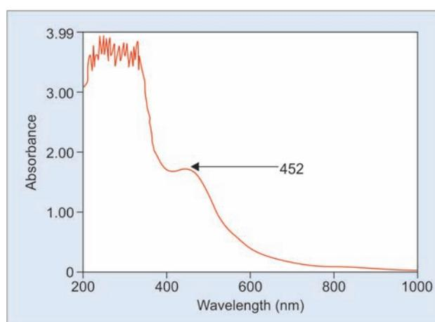
**Graph 1:** UV-visible absorption spectra of synthesized cerium NPs showing peak at 452 nm
