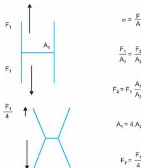
Fig. 6: Reduced contact results in reduced physical stress
