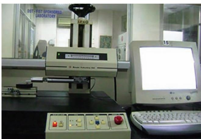
Fig. 7: Three-dimensional optical profilometer
