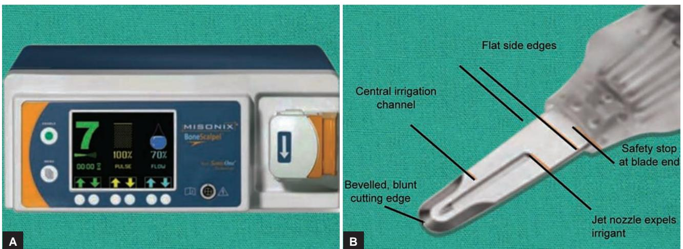
**Figs 1A and B:** Ultrasonic bone scalpel device and its tip view
