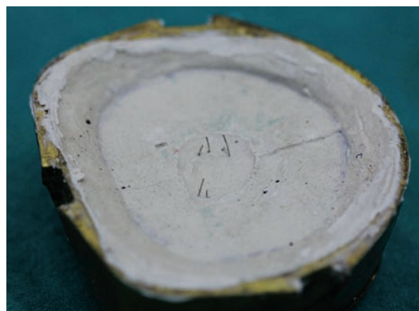
Fig. 5: The wire pieces attached to the posterior portion of the mold after dewaxing
