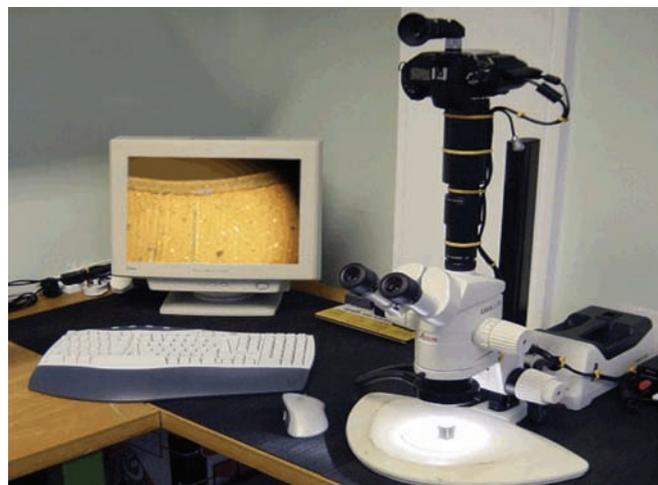
**Fig. 2:** Stereomicroscope
