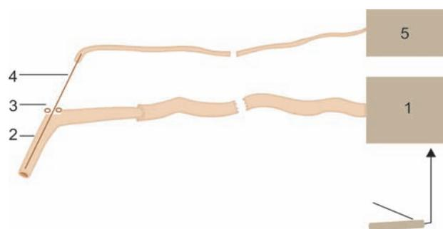
**Fig. 1:** Principle of operation of the device for removal of cyst's contents accepting capacity; 1 – the accepting capacity for remote contents of a cyst; 2 – bent tube; 3 – lateral aperture; 4 – needle for puncture; 5 – source of vacuum
